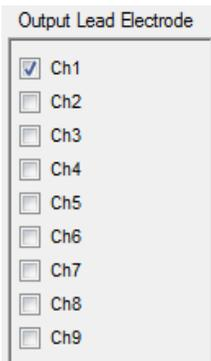
This section allows the user to select which lead electrode the output is connected to (i.e. terminal P1 in the IEC 80601-2-26:2019, Figure 201.104). Unselected electrodes are connected to the system ground (terminal P2 in Figure 201.104).
