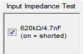
This check box allows the user to switch in an impedance of 620kΩ/4.7nF in series with the main function, for testing the input impedance of the EEG device under test. When the check box is ticked, the impedance is shorted. The ±150mVdc offset can be used in conjunction with this test.
