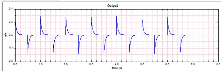
The output display provides an image similar to that provided by EEGs. The sensitivity of the display range may be set at 0.1mm/μV, 0.05mm/μV or 0.02mm/μV to cover the full range of waveforms offered by the system. The time rate is fixed. The output display uses the same data as used in the DAC output and serves as a cross check of the selected waveform.
